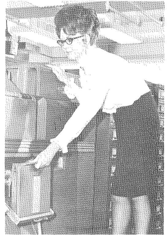
Doris Walters inserts panel into 519 Reproducer where mark-sensed clock cards are translated into punched holes for further processing.
