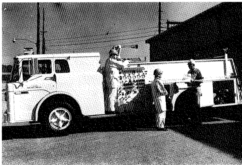
NEW PUMPER — Chief Ora Tussey (right) checks out equipment on new fire pumper with firemen George Cooke (left) and George King (center). The new apparatus was placed into service at the GAT Fire Station in October. It has a pumping capacity of 1000 gallons per minute and a 300 gallon water tank.
