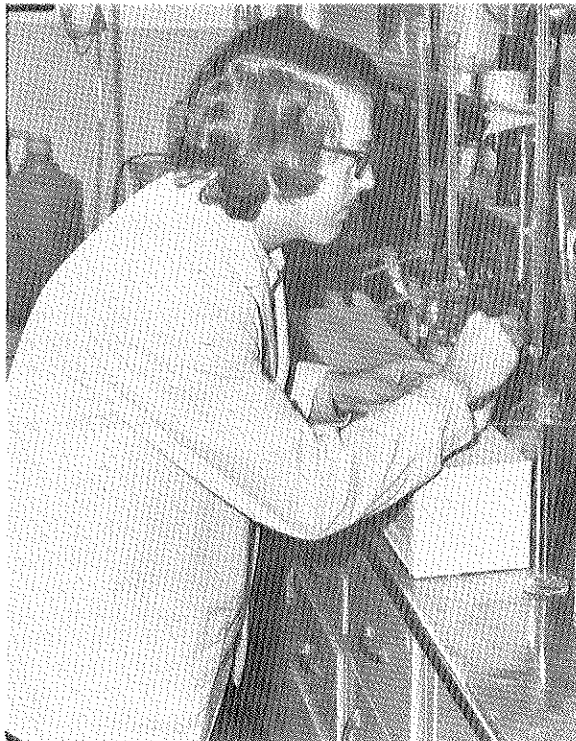
LARRY LITTON, chemical engineering major from West Virginia Institute of Technology, titrates a plant water sample for total hardness in Process Laboratory of Chemical Operations.
