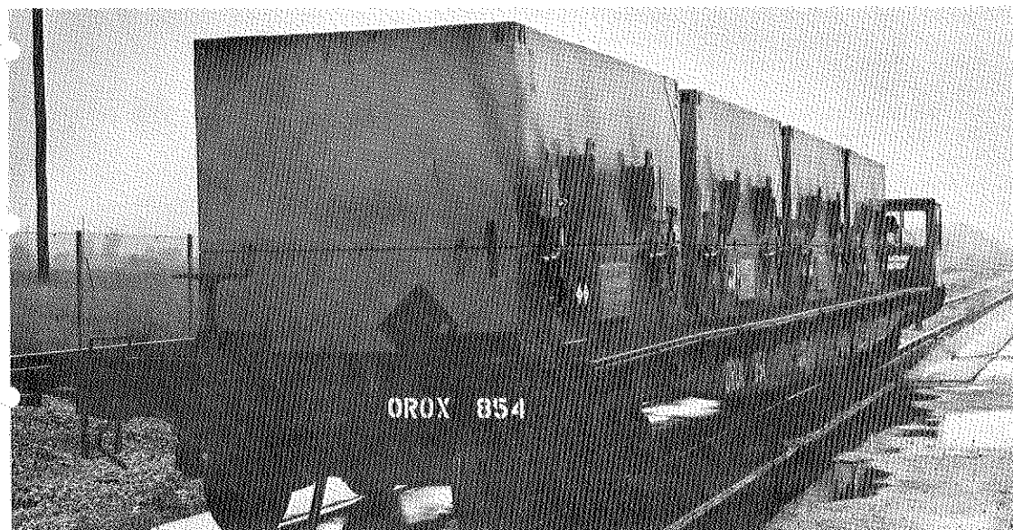
NEW SYSTEM. A newly designed UF6 packaging and transporting system moving into unloading dock at X-344 Bldg.
