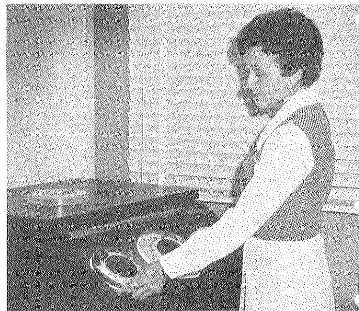
ELOISE THOMAS removes converted data, in magnetic tape form, from Inforex System. This data is then read directly by the computer.
