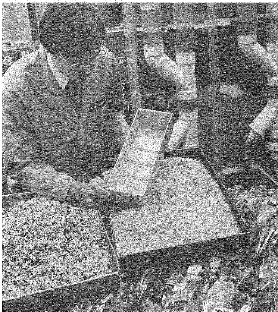
Polyester chips reclaimed by processing empty soft drink bottles through Goodyear's new pilot plant in Akron are compared with chips before processing (left tray) and a drawer made from the recycled material. Goodyear built the low-cost facility to illustrate the relative ease of reclaiming polyester from the lightweight, shatter-resistant bottles.
