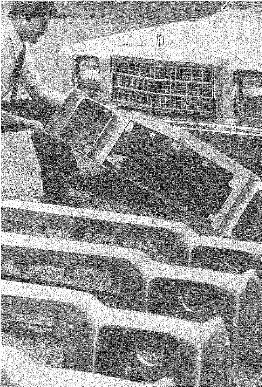
Plastics in cars mean less weight and better gas mileage. Reinforced plastic parts like these grill and headlight panels produced by Goodyear's Jackson, Ohio, plant for the Ford Granada could account for up to 500 pounds of a car's weight by the mid-1980's -- nearly double the plastic used in today's typical passenger cars.
